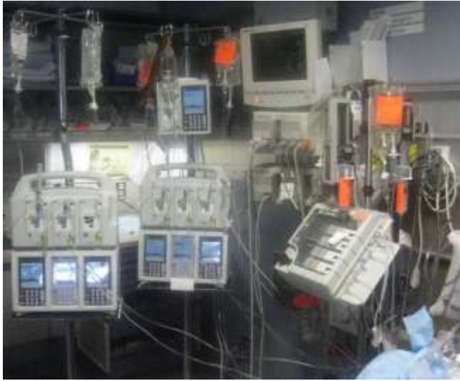
Figure 10: Actual IV Line Set-Up for a Patient Receiving 15 Infusions
