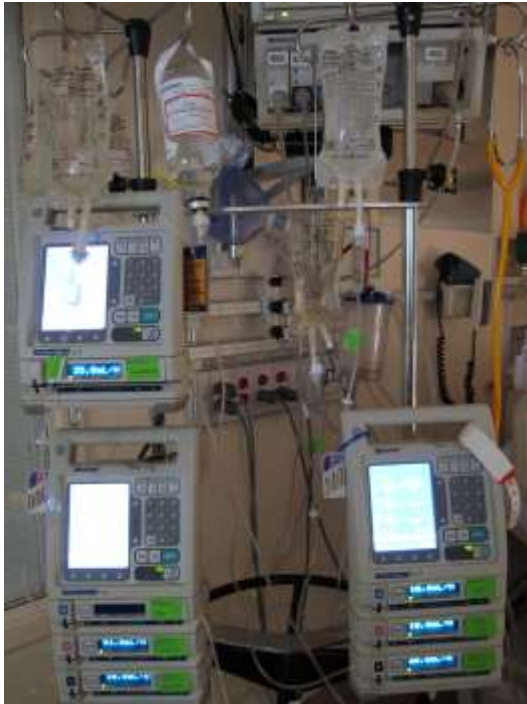
Figure 12: Confusing Proximity Between IV Bags and Pump Channels
